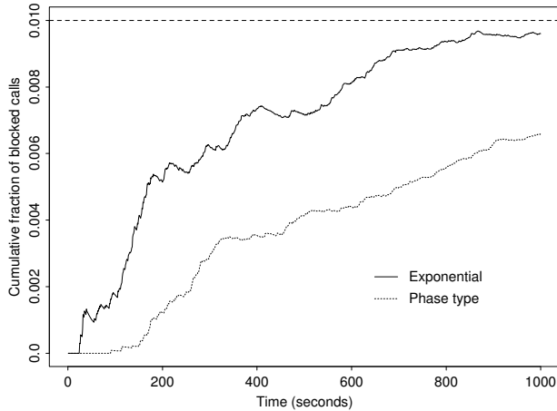
Figure 10: Comparison of simulated cumulative fractions of blocked attempts shows that uncongested periods are also relatively more persistent in the presence of long holding times. Here two systems of 96 access circuits, both starting with only 81 busy circuits, are compared. Note that for the phase type model with long holding times, the observed blocking rates are consistently below the one for the comparable exponential model.
